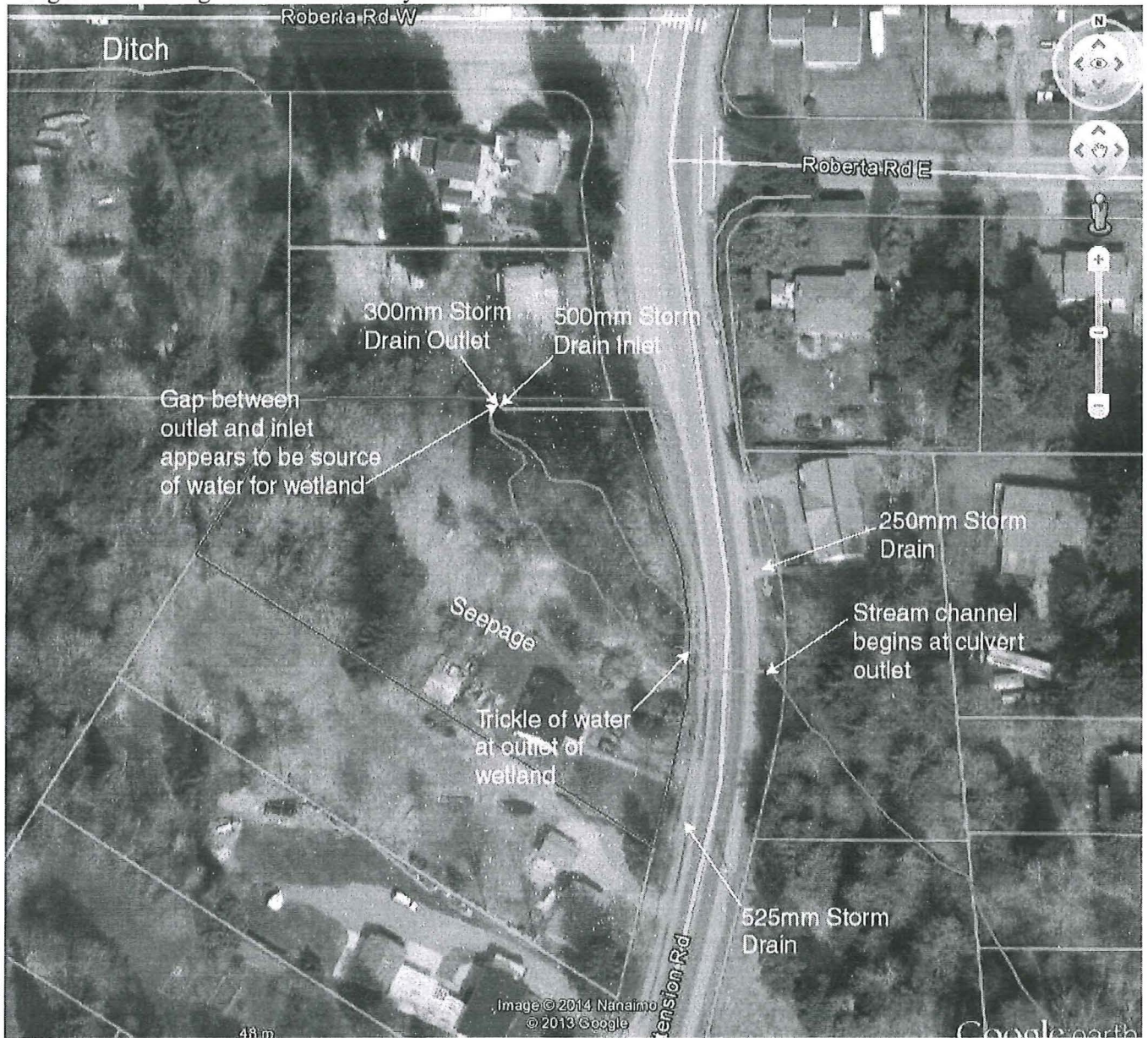
Figure 2. Drainage and storm drain systems associated with 1601 Extension Road
